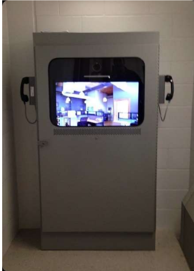
Figure 1. Correctional Video Unit with the Privacy Phone
